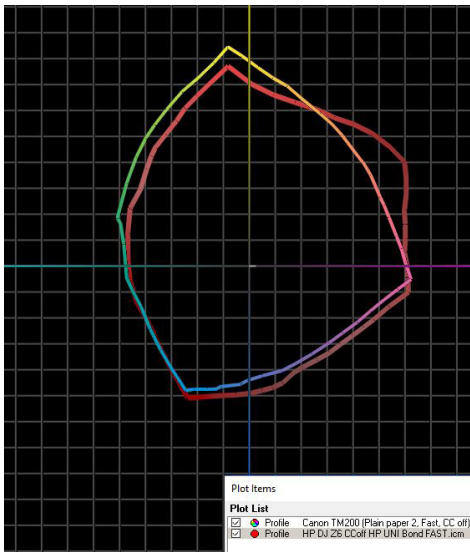
Canon imagePROGRAF TM-200 colour gamut on plain paper in Fast settings (shown chromatically) versus HP DesignJet Z6 colour gamut (shown in red) on plain paper in Fast settings.
